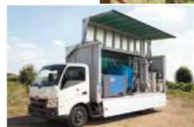
Mobile Ceramic Membrane Filtration Equipment
