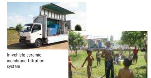
In-vehicle ceramic membrane filtration system
